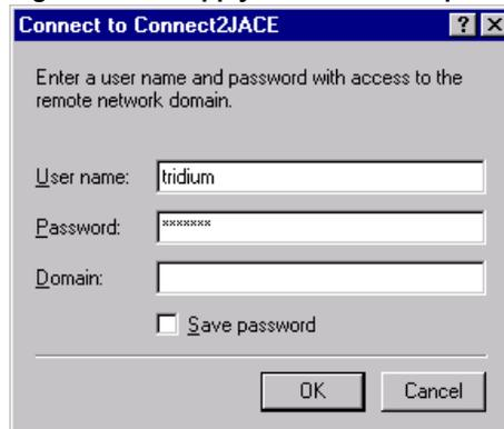
RAS attempts to establish a connection between the modem on your computer and the modem on the remote host. Wait for the connection to be made.
